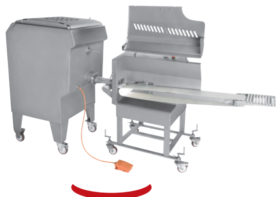
Raccordement TX32ML + Portio 140 (en position nettoyage) Connecting TX32 ML + Portio 140 (in cleaning position)
