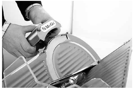
Fig. 6 Extending the sharpener from the arbor
