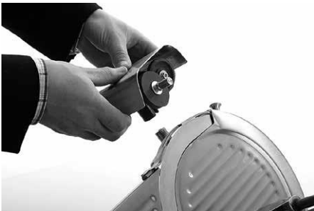
Fig. 7. Preparing for sharpening
