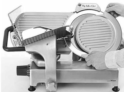
Fig. 9. Removing or attaching the knife cover
