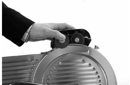
Fig. 8. Sharpening the knife
